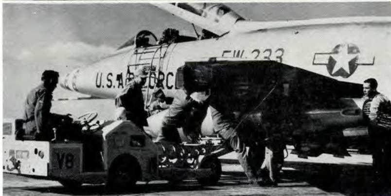
Ground crewmen install equipment for refueling mission by an F-100 tanker.
