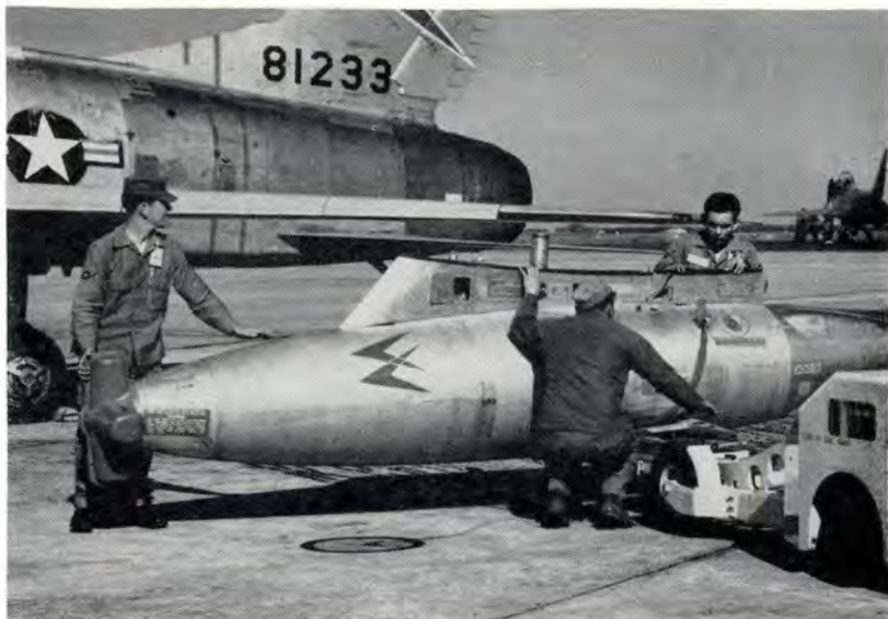
A loading team eases a special 300-gallon tank under the wing of an F-100 tanker.
